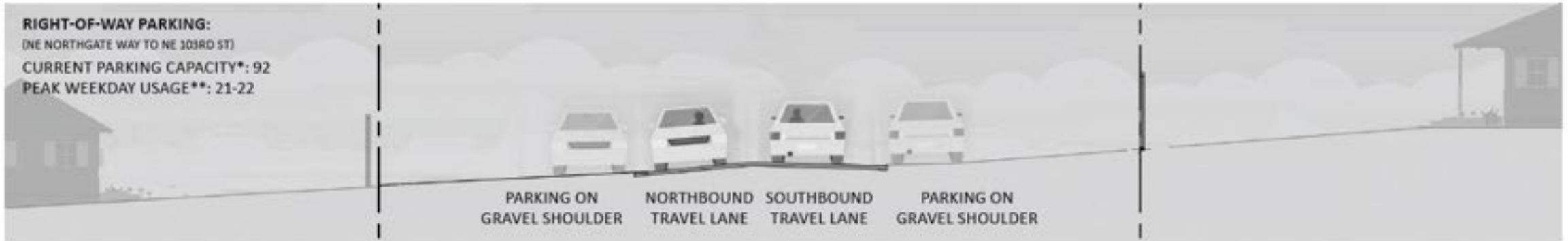
EXISTING TYPICAL STREET SECTION WITHOUT DITCH 23RD AVE NE
